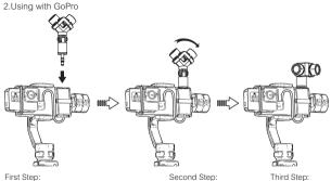
Insert microphone into 3.5mm TRS socket
